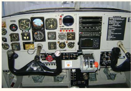
In addition, electronic digital gauges (ITT, N<sub>1</sub>, N<sub>2</sub>, oil pressure, oil temperature, volt and ammeter, torque, fuel pressure/fuel flow), gascolator, power quadrant and baffling kit were fitted.
